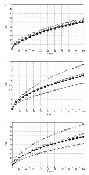
FIGURE 1. Flow curves of 20 g/L potato starch dispersions gelatinized in the presence of 20 g/L ---, 40 g/L ---, 60 g/L --- kaolin and without kaolin ---, measured before (a) and after 24 h (b) and 48 h (c) storage.
