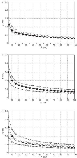
FIGURE 2. Viscosity flow curves of 20 g/L potato starch dispersions gelatinized in the presence of 20 g/L --, 40 g/L --, 60 g/L -- kaolin and without kaolin --, measured before (a) and after 24 h (b) and 48 h (c) storage.
